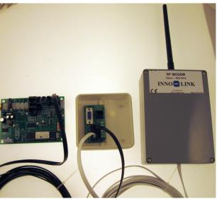
The cable from the Slave is connected to the Connection box for Pole, and a cable is connected from the Connection box pole to the Sign controller or the Combi controller. The cable from the Slave can also be connected directly to the Combi controller.
