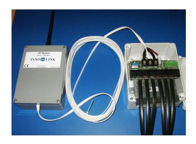
For rollerblinds, the cable from the slave is connected to the plug in the middle in the power supply.
